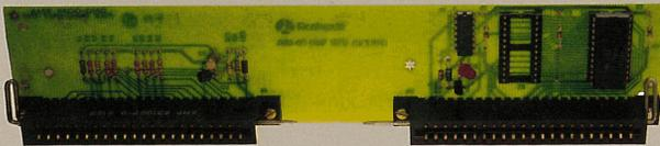
For the OEM, the AIM 65 Self-Test Module and Manual are valuable additions for maintenance and service. The module includes ROM-based software which performs individual tests, all tests, or repetitive tests of the installed ROMs, RAMs, and other MOS devices. Service and fault isolation procedures are included for the peripherals as well as the microcomputer module.
