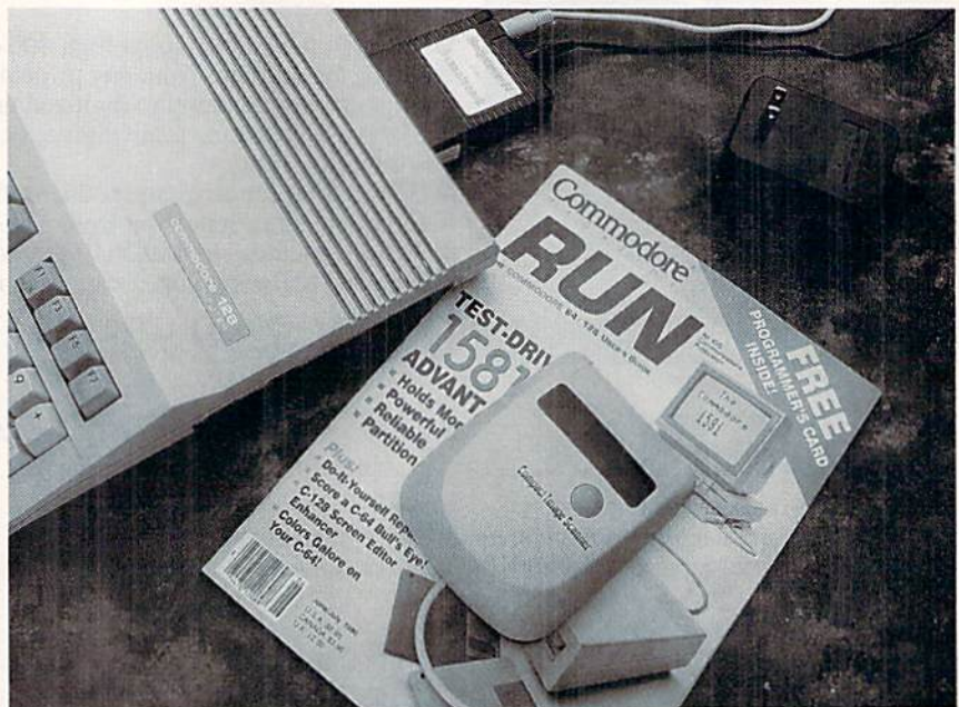
The Handyscanner setup: An auxiliary power supply and the scanner both plug into a cartridge in your computer's user port.
