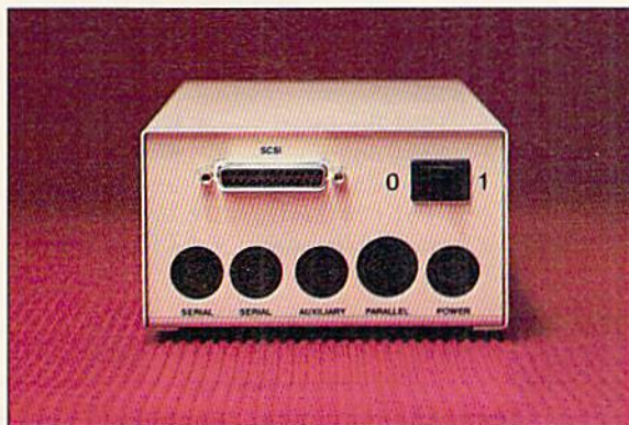
Rear view of HD-40 displays the drive's many ports.
