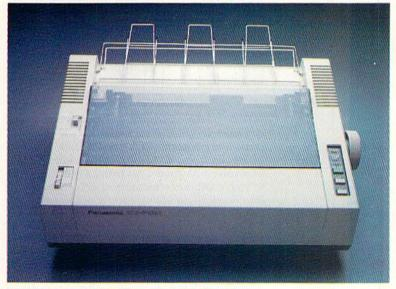
Panasonic's KX-P1091 dot matrix printer features NLQ, Draft and Compressed modes.
