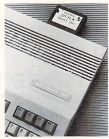
The Double Quick Brown Box plugged into the C-128's expansion port.
