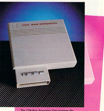
The 1750 Ram Expansion Unit increases the C-128 by 512K, for a total of 640K.
