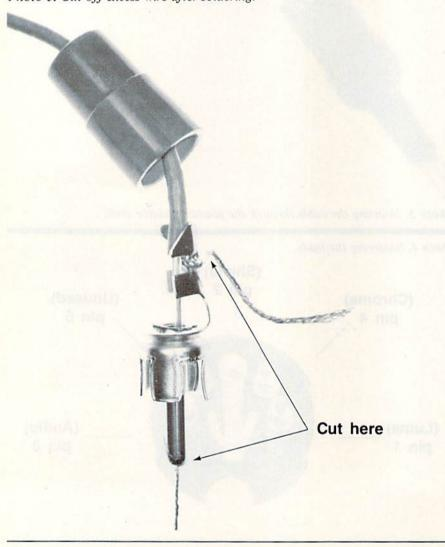
For an improved display, all you need are a soldering iron and access to a Radio Shack store that the large opening is facing the unsoldered end of the cable. Likewise, slip the white insulator over the cable soldered to pin #3 and the red insulator over the cable soldered to pin #4.
