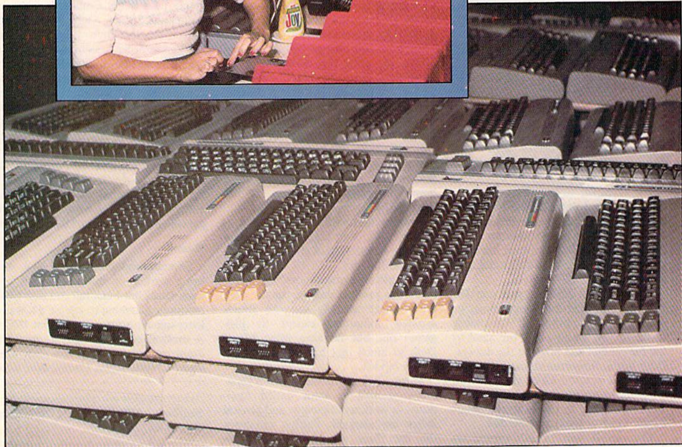
Pallets of completed and checked C-64s en route to conveyor for packaging.
