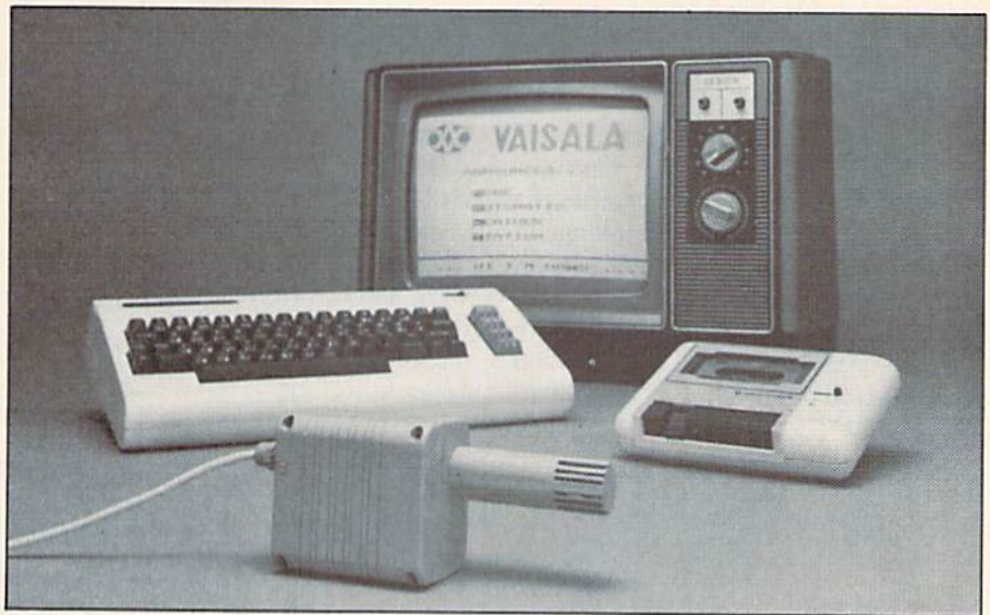
Vaisala's Home Automatic Weather Station.
