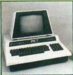
*Chuck Peddle designed and developed the Personal Computer. The machine should be immediately operational after plugging it in. The result was the PET. Nearly the same time the Apple II appeared. The PET was characterized through: build in monitor, integrated cassette device and the well-known BASIC interpreter by Microsoft. The PET had many revisions to endure and is still popular. In particular, it was converted up to have an adequate and thus understandable typewriter keyboard.*
