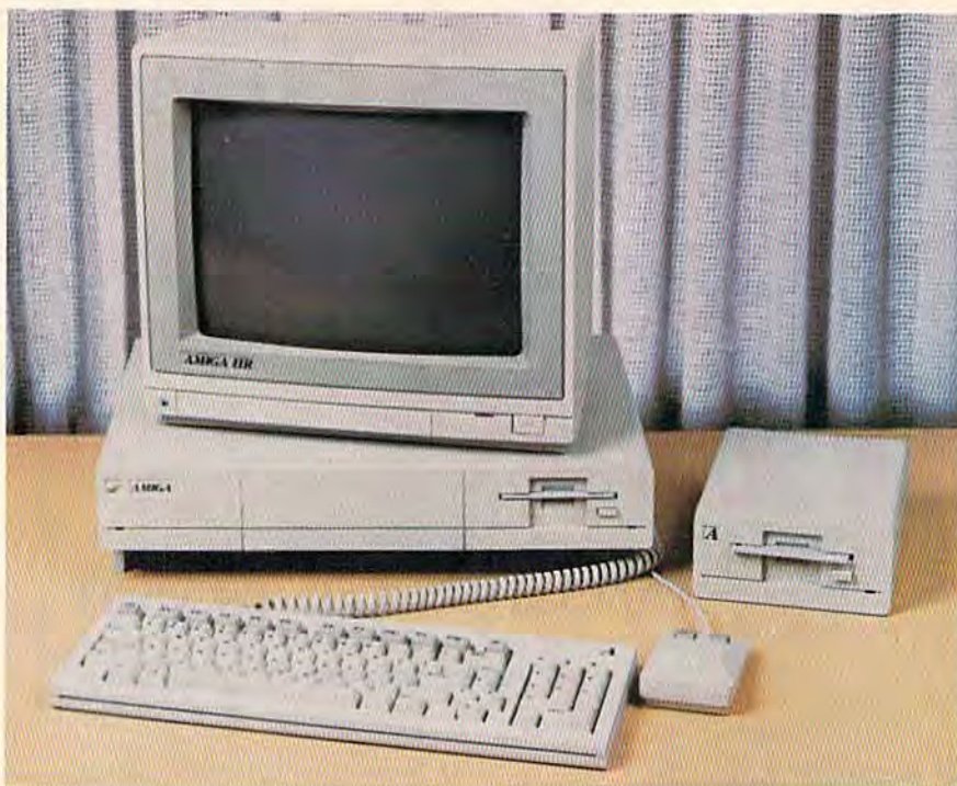
The Amiga computer from Commodore, with built-in 3½-inch disk drive, detached keyboard, two-button mouse, and optional RGB monitor, and external drive.
