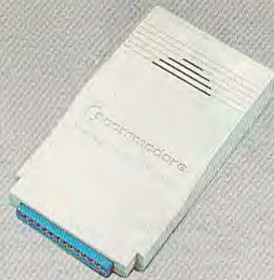
The 1670 modem from Commodore features 300/1200 baud, built-in speaker, auto answer, autodial, auto baud, and auto mode selection.
