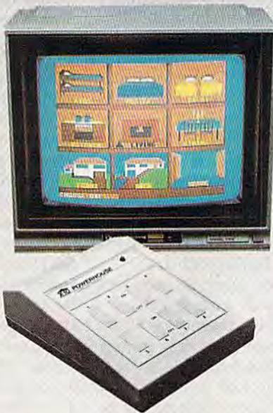
The X-10 Powerhouse, a programmable interface for the 64, allows control of household lights and appliances without tying up the computer. The accompanying icon-based software lets you simulate the layout of your home and program individual rooms or outside lights.
