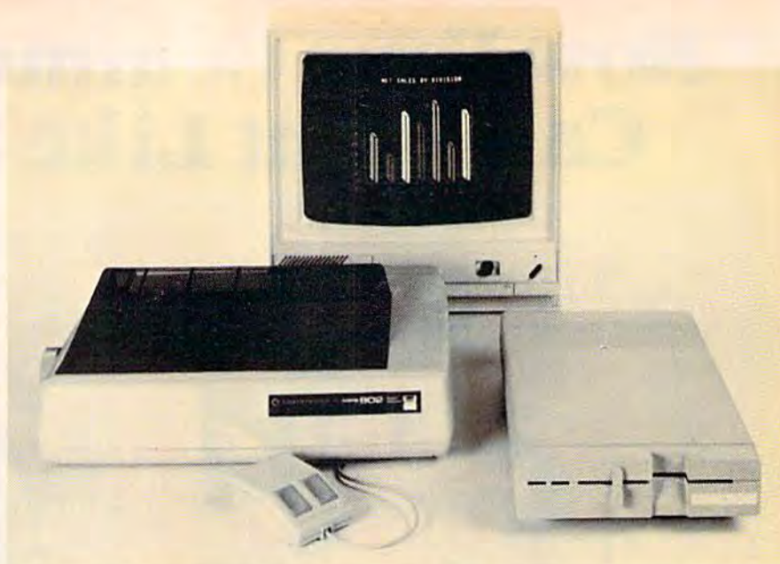
Among the new Commodore peripherals are the Mouse, MPS 802 Printer, 1902 RGBI/Composite Monitor, and the 1571 Disk Drive.
