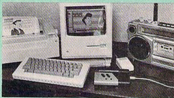
The Shuttle Communicator can download information from a radio station to any home computer, at speeds of up to 4800 baud.
