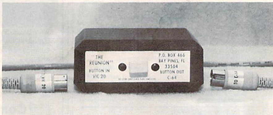
The Reunion, by Hytech, simultaneously interfaces the VIC-20 and Commodore 64 with a disk drive and/or a printer, providing two computer systems.
