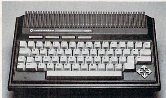
Commodore's new 264 computer, showing the four separate cursor keys (lower right) and the four programmable function keys (at left above keyboard). The Commodore 364 will have a similar console, but with a 19-key numeric keypad above the cursor keys.
