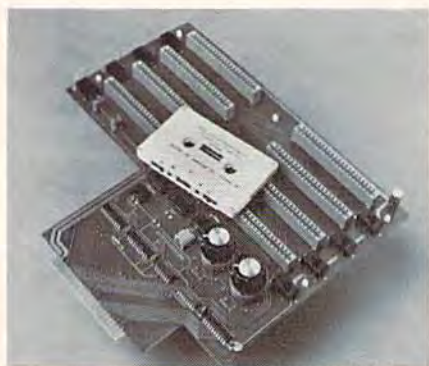
Compuscope's Supermother provides eight expansion slots for the VIC.
