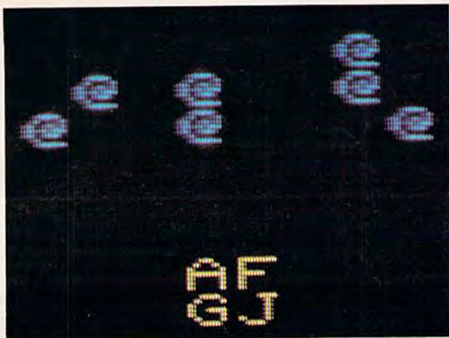
A close-up screen photo showing how ordinary characters (left) are transformed into custom characters (right) for the VIC-20 version of "Chicken Little," a game program elsewhere in this issue. Note the technique of combining one or more characters (A, F, G, J) to form a single, large custom character.
