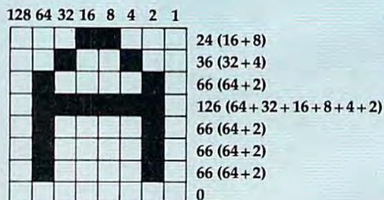
Figure 3: Dot Pattern For A On VIC-20
