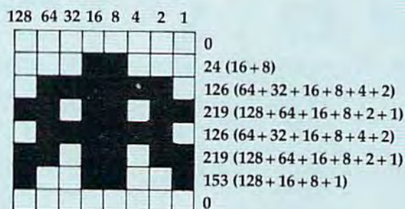
Figure 4: Dot Pattern For A Customized Character (Space Invaders-Type Alien)
