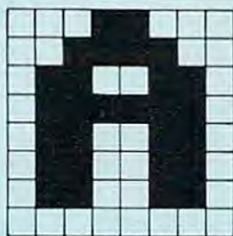
Figure 1: Dot Pattern For Character A On Commodore 64
