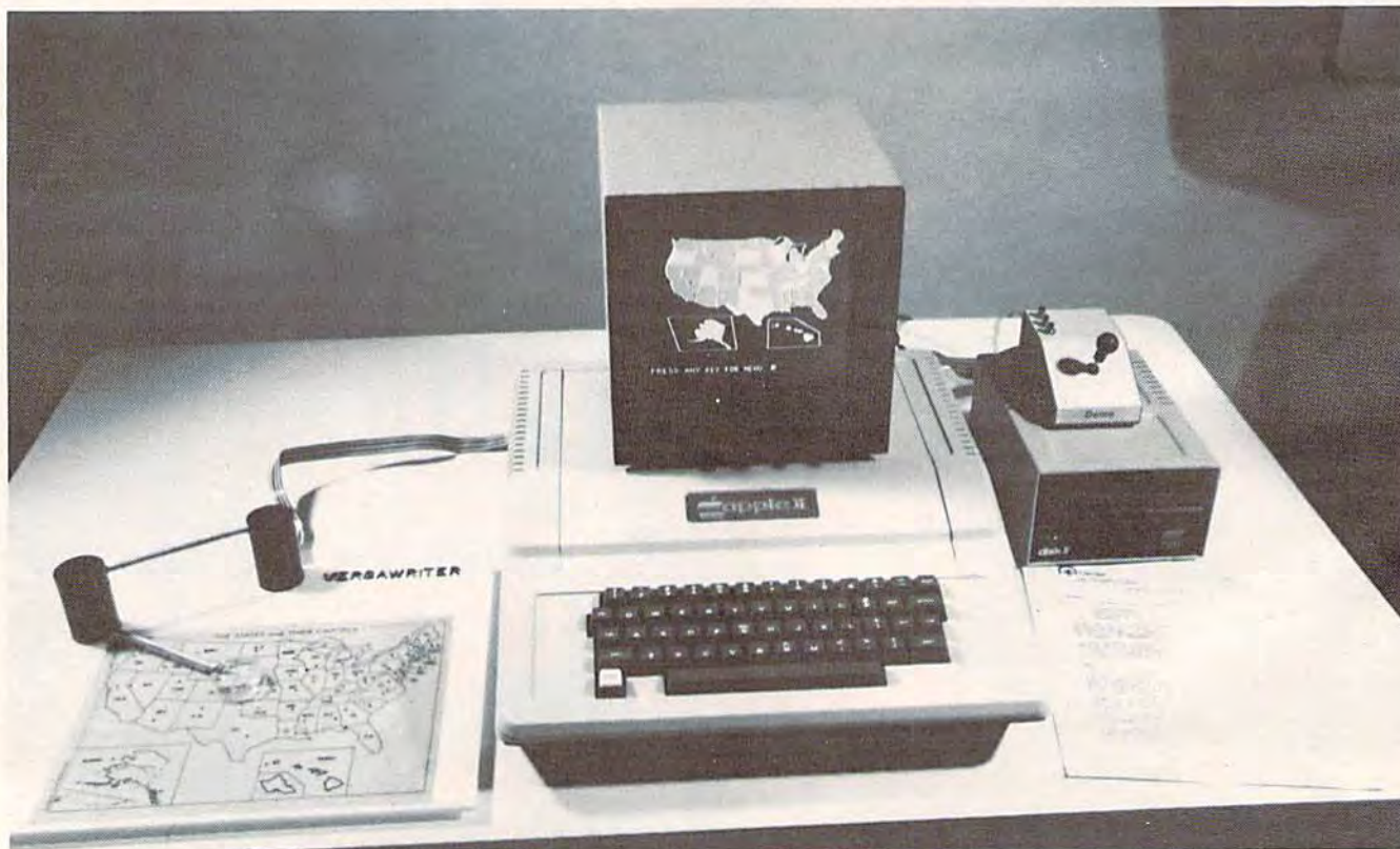
With a graphics tablet, you can copy maps, photographs, or diagrams into the computer by tracing them with the graphics arm wired to the computer. (Courtesy of Versawriter Inc.)
