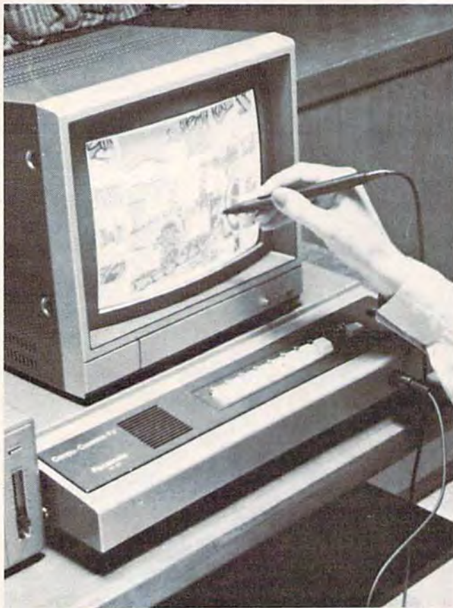
Drawing pictures directly on the TV screen with a light pen. (Courtesy of Matsushita Electric.)
