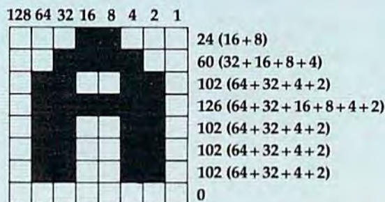
Figure 2: Dot Pattern For A On Commodore 64
