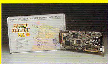
'SOUND GALAXY NX PRO 16' supports the 5 most popular sound cards. Features CD ROM interface, 16 Bit stereo playback with 20 voices at up to 14.4 KHz, volume control, midi interface, game port, 4 watt amp, and software setup. $169
