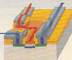
How a transistor operates as a switch.
