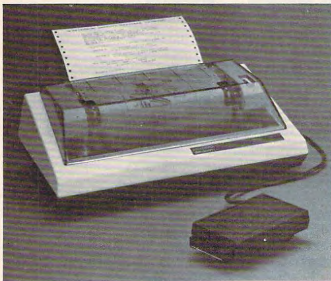
Axiom's $299 dot matrix printer with dot-addressable graphics is plug-compatible with the TI-99/4A.
