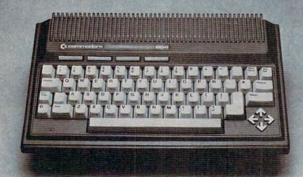
The Commodore 264. Note the unusual arrow-shaped cursor keys. The Commodore 364V is similar, but has a numeric keypad to the right of the keyboard.
