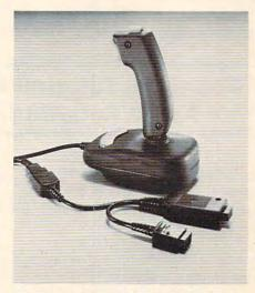
The TI version of the Competition Pro 3000 joystick includes an adapter for the TI-99/4A computer.
