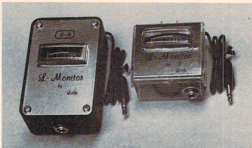
The L-Monitor, a microammeter used to improve transfer of data to or from cassette tape, comes in an assembled version, left, or in kit form.
