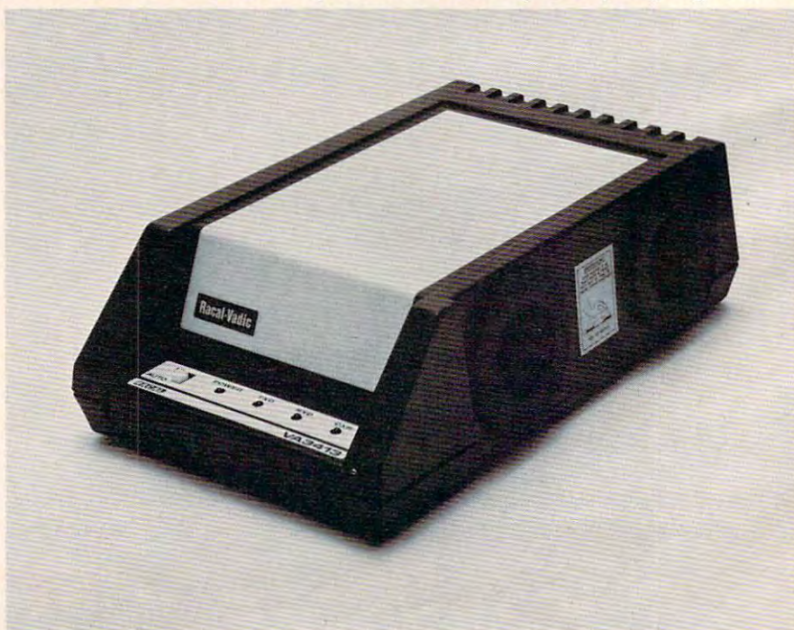
The Racal-Vadic VA3413 is an acoustic modem. The telephone handset is pushed into the soft rubber cups on the side.
