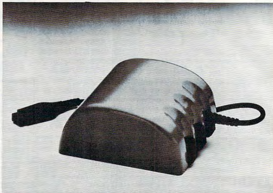
Wico's Command Control Mouse is an optically encoded mechanical cursor control.
