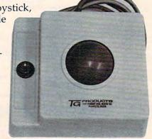
ball glides less smoothly than the WICO's, however, and has much less tendency to coast. Approximately one third of our testers preferred this "feel" for fine positioning, so this is purely a personal matter that should be tested by the purchaser. Inside, the TG Trackball supports the "billiard ball" on plastic shafts without ball bearings. It might be a good idea to lubricate these shafts to reduce excessive wear if this hasn't been done in production models.
