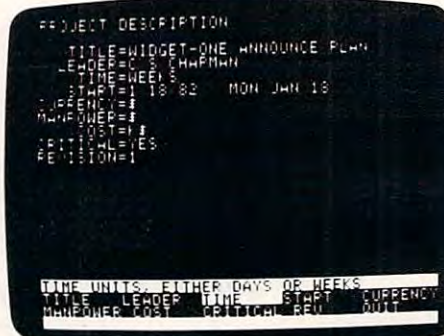
The Modify Menu allows the user to create or change the overall description of the project. Such items as title of project, leader, currency, cost levels and revision number can all be changed. Modify is where the user sets up manpower, skills, costs, holidays and the work week. The moving cursor anticipates the next entry so that keyboarding time is reduced.
