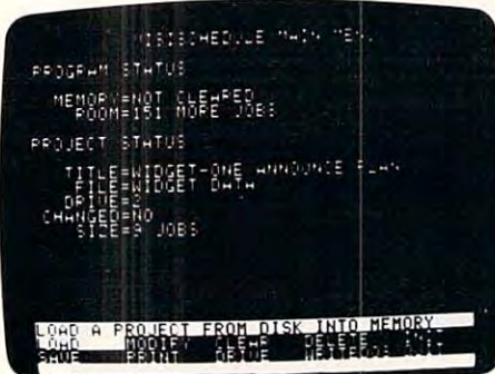
The VisiSchedule™ program automatically loads details from the previous use of the program. The user can re-load a project schedule already set up, or create one from scratch. Current date, person preparing report, current status of last project worked on can be checked.
