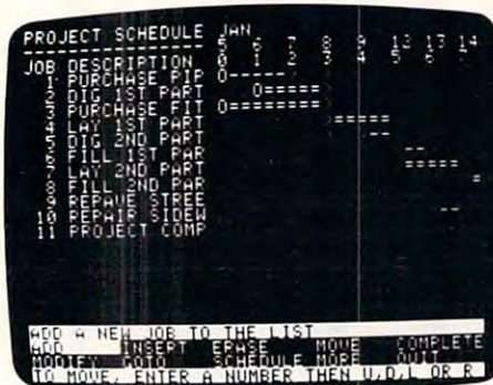
This displays the work schedule itself. The user may scroll in all four directions to view the entire project. Simple menu commands add, delete or rearrange jobs. As each job is entered, it is displayed on screen. Once jobs are entered, manpower peaks may be auto leveled, costs and manpower levels are displayed or the project schedule adjusted in many ways.
