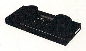
The Cat and D-Cat have been specially prepared by Skyles for interfacing to the PET user port (not to the IEEE port) and with a special cassette program, allowing communication
