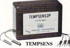
This module provides two temperature probes for use by the AIM16. This module should be used with the MANMOD1 for ease of hookup. The MANMOD1 will support up to 16 probes (eight TEMPSENS modules). Resolution for each probe is 1°F.
