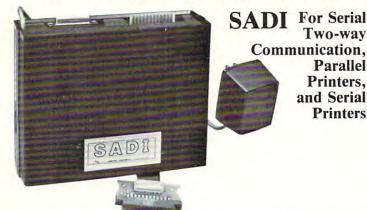
SADI - The microprocessor based serial and parallel interface for the Commodore PET. SADI allows you to connect your PET to parallel and serial printers, CRT's, modems, acoustic couplers, hard copy terminals and other computers. The serial and parallel ports are independent allowing the PET to communicate with both peripheral devices simultaneously or one at a time. In addition, the RS-232 device can communicate with the parallel device.
