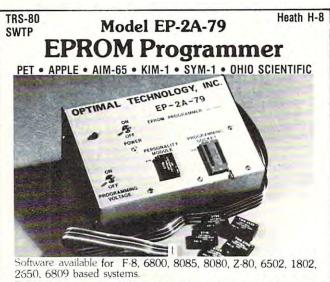
EPROM type is selected by a personality module which plugs into the front of the programmer. Power requirements are 115 VAC 50/60 Hz, at 15 watts. It is supplied with a 36-inch ribbon cable for connecting to microcomputer. Requires 1<sup>1</sup>/<sub>2</sub> I/O ports. Priced at \$169.00 with one set of software. (Additional software on disk and cassette for various systems.) Personality modules are shown below.
