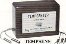
This module provides two temperature probes for use by the AIM16. This module should be used with the MANMODI for ease of hookup. The MANMODI will support up to 16 probes (eight TEMPSENS modules). Resolution for each probe is 1°F.
