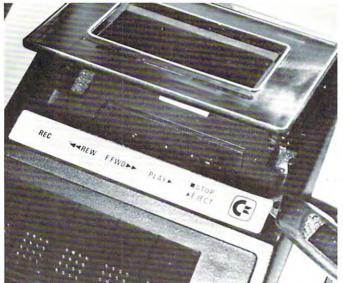
Figure 2 - To get at the screw hole in the push-button-eject model you must remove the metal label strip as shown.
