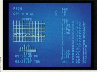
ABOVE: Microtroll's immediate mode screen display. Digital oscilloscope screen is to the left; monitoring of the 16 channel analog to digital convertor is on the right.
