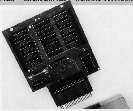
The SSI00 Plus' cartridge expansion socket facilitates use of a ROM or EPROM cartridge for control applications.
