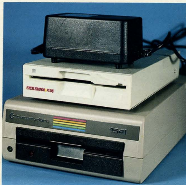
Top: FSD-2 and its power supply atop the 1541. Middle: bottom view, showing direct drive TDK module, 6502 microprocessor, two 6522 VIAs, 16K of ROM, 2K of RAM, and DIP switches. Bottom: top view, showing remaining circuits. READER SERVICE NO. 167
