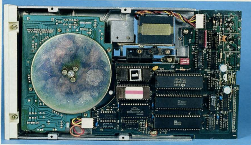
Top: FSD-2 and its power supply atop the 1541. Middle: bottom view, showing direct drive TDK module, 6502 microprocessor, two 6522 VIAs, 16K of ROM, 2K of RAM, and DIP switches. Bottom: top view, showing remaining circuits. READER SERVICE NO. 167
