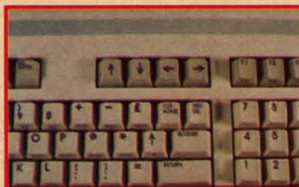
Above the main keyboard of the 128 are (top) Esc, Tab, Alt, Caps Lock, (middle) Help, Line Feed, 40/80, No Scroll, and (bottom) cursor keys.
