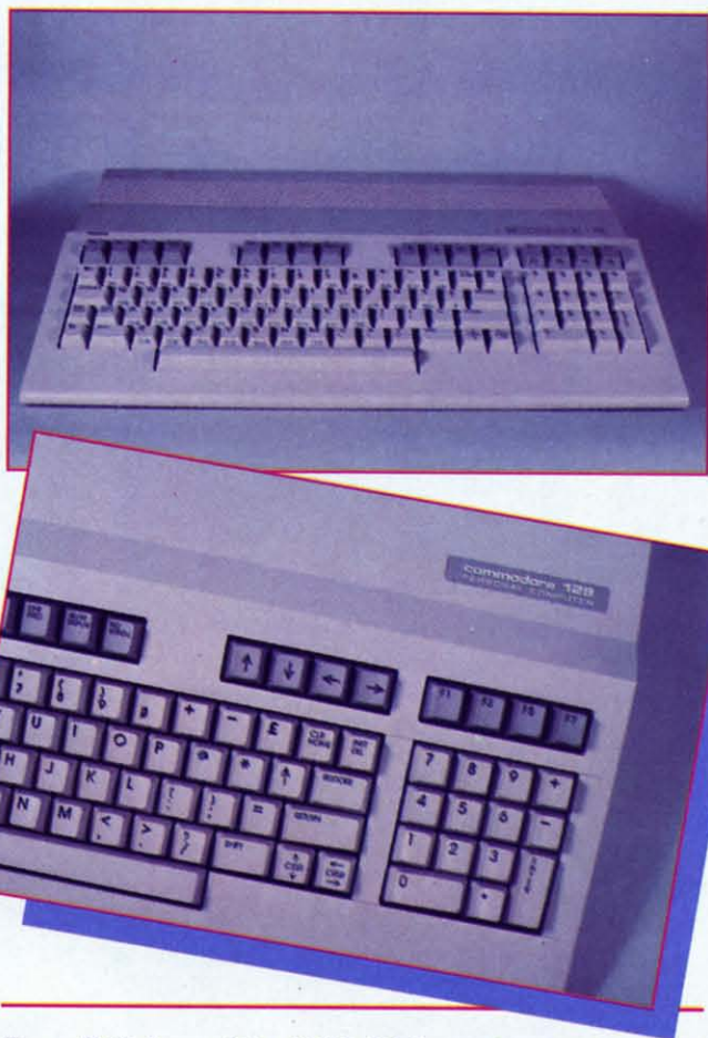
Top: all 92 keys of the C-128. Main section nearly duplicates the C-64. Bottom: closeup showing numeric keypad.
