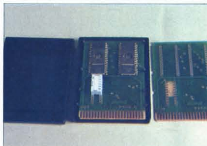
A Cartridge-Maker-64 cartridge. Center: EPROMs installed. Right: bare.
