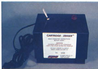
The built-in ultraviolet light source allows you to erase your EPROMs.
