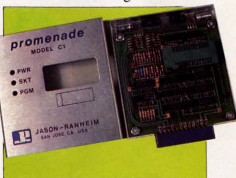
The Promenade inside and out. The 4 x 5" package installs in user port.
