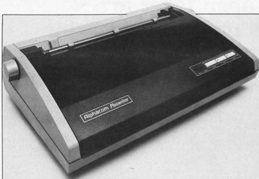
The Alphacom Pluswriter (see review on page 66) cruises at a moderate 18cps. The printer emulates the Diablo 630, so many special effects are possible. READER SERVICE NO. 265
