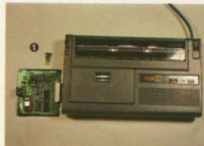
The Okimate 10 Color Printer, side by side with its attendant ① user-replaceable thermal print head and ② Plug 'n Print module. READER SERVICE NO. 268
