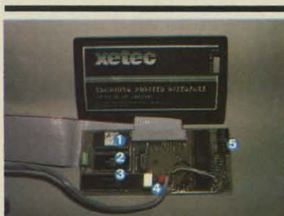
Inside Xetec GPI: ① 4K interface ROM; ② 2K RAM buffer; ③ 6802 microprocessor; ④ interface clock crystal; ⑤ setup switches
