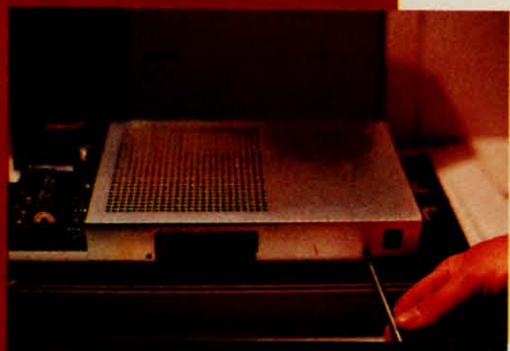
Removing two Phillips screws that hold on chassis cover.
