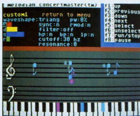
ADSR screen of ConcertMaster lets you use function keys to control attack, decay, sustain, and release. READER SERVICE NO. 259
