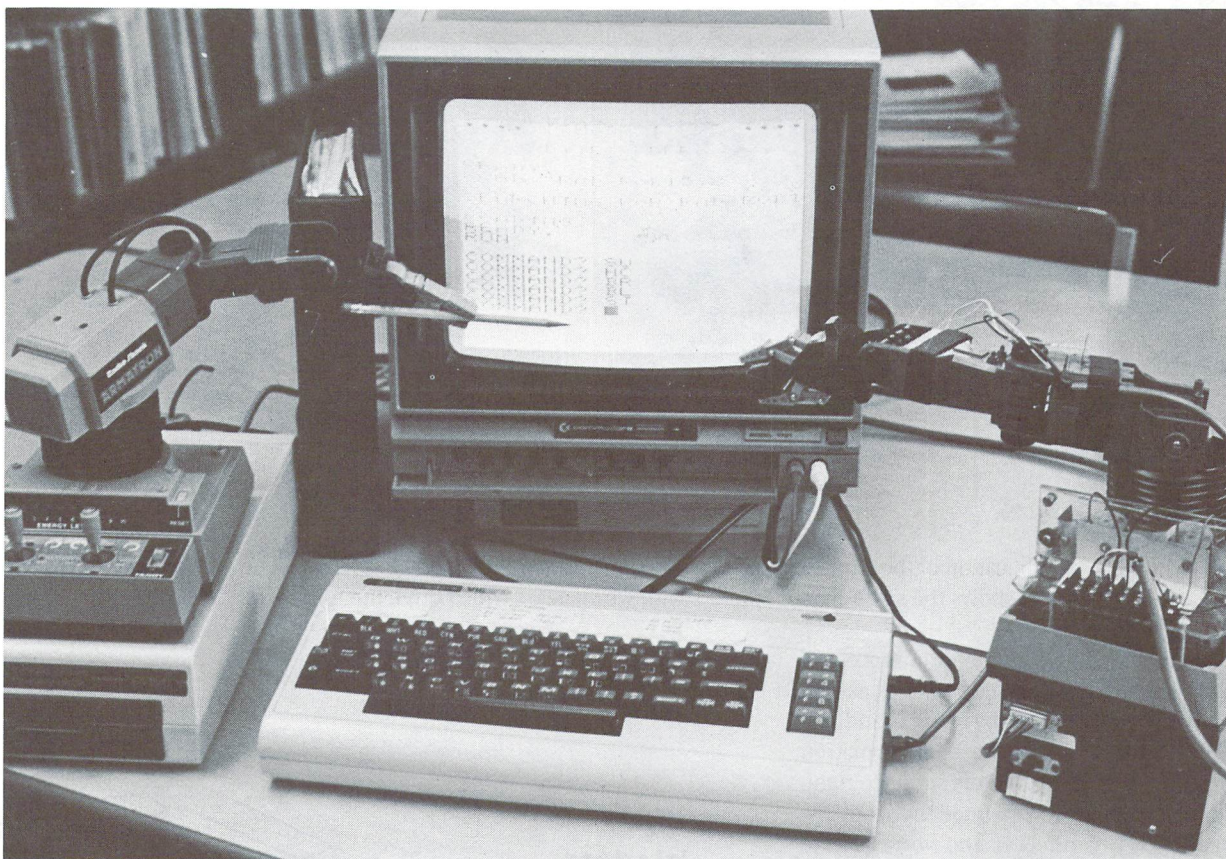
Figure 1. Armatron Robot Arms. The left model on top of the disk drive is unmodified and shows the two joysticks for control. At right the modified robot arm sits on top of the power supply and interface box.
