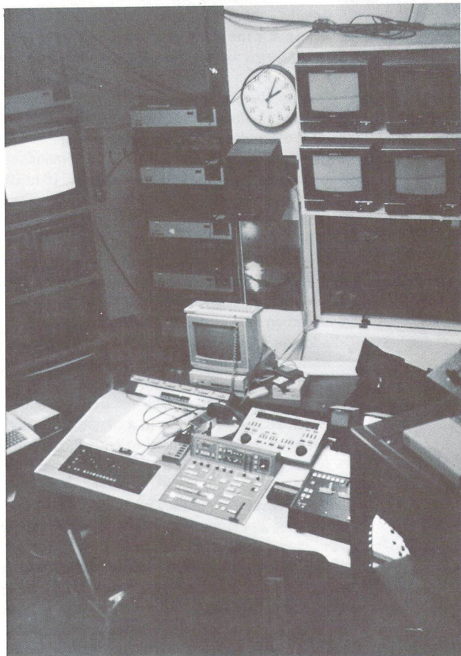
The control room of the Amiga Studio Theatre: the foreground controls are for switching and special effects, while the Amiga in the background is reserved for the TheatreSports event.
