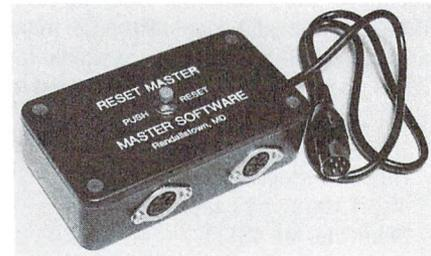
Reset Master simply plugs into any serial port on your computer system, and therefore is installed without opening the computer case and without any soldering. Rather than just shorting the computer's reset signal line to ground, Reset Master contains electronic circuitry to protect your computer.
