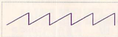
Figure 5. A sound created with the Sawtooth waveform.
