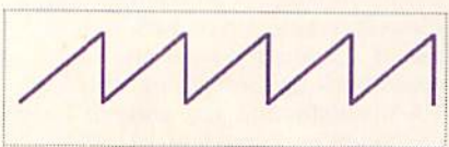
Figure 3. The Sawtooth waveform.
