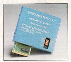
The Turbo Master CPU features easily accessible DIP switches.
