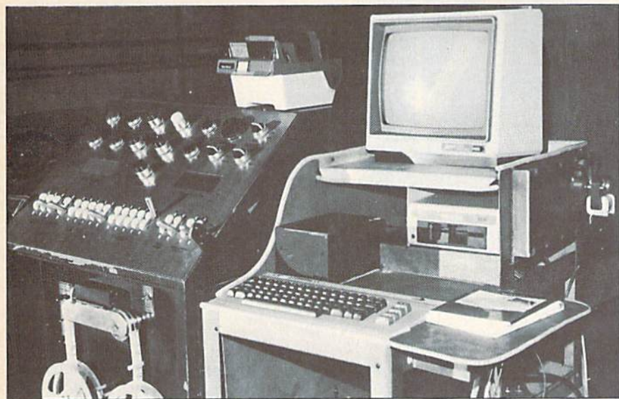
C-64 interfaces with milling machine to streamline production.
