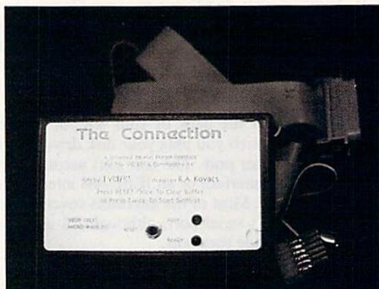
On the positive side, this interface may be used not only for an RS-232 printer, but also for an RS-232 modem or other peripheral device. It is also possible to manually open up a data transmission channel to the user port via a short program (consult your programmer's reference guide for details), but this, once again, may conflict with the applications software you intend to use.
