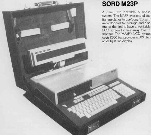
system. The M23P was one of the first machines to use Sony 3.5 inch microfloppies for storage and also one of the first to have a workable LCD screen for use away from a monitor. The M23P's LCD option costs £500 but provides an 80 char-
