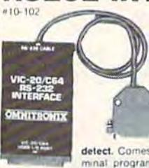
Connects to the User port and provides full RS232 signals for modems and printers. 2 foot cable with male DB25 connector. Supports full complement of RS232 signals including Ring detect. Comes with a type-in BASIC terminal program and printer hook up instructions.
