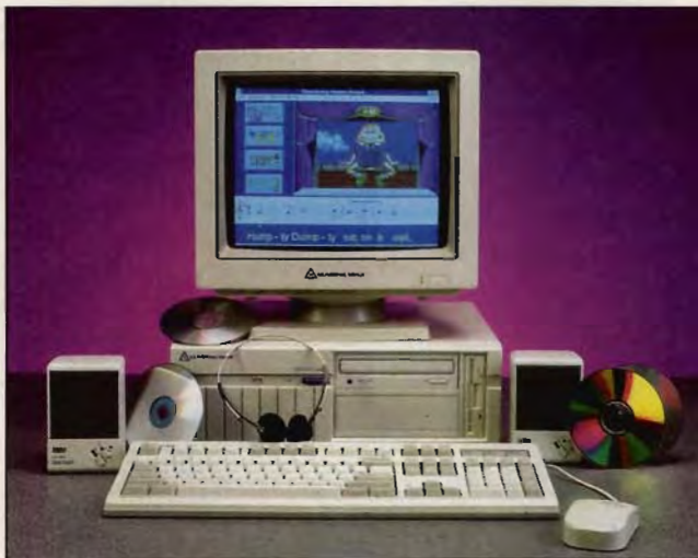
With a 66-MHz CPU, VESA local-bus graphics, and double-speed Sony CD-ROM drive, the WinPro is fast and powerful.
