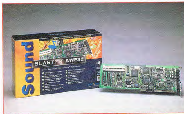
The Sound Blaster AWE32 features a new E-mu Systems DSP chip.
