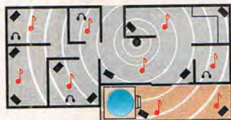
Recoton's transmitter sends music through walls to wireless speakers over a 75,000 square foot area.
