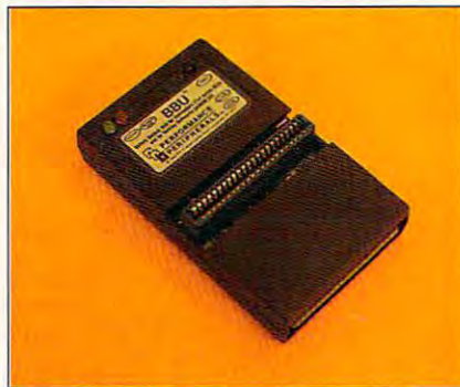
BBU is a battery backup interface module for 1700-series REUs and geoRAM 512.
